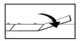
Continue along the wall until you reach the last full plank, connecting each plank in manner described above. To fit the last plank, turn plank over (face down). Place the plank in the corner so the tongue on the short end touches the adjacent wall. Measure overlap between the installed plank and the last plank.
